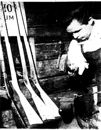
GUNSMITH RALPH MARCUM, SAND GAG HAMMERS A TRIGGER GUARD INTO SHAPE as he makes a flintlock rifle similar to the one Daniel Boone used. Marcum is part of the Kentucky Guild of artists and Craftsmen exhibit at the Kentucky State Fair, August 14-23 in Louisville.
