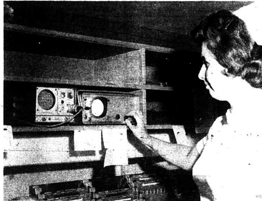
Mrs. Jenay Payne, LPN, is shown with the Electrocardiographic monitoring machines which allow a constant observation of patients in the cardiac care unit by nurses at the nursing station.
