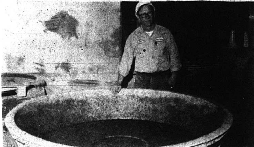
DeAlva Russell, in charge of the fiberglass section, is shown with one of the forms used to manufacture fiberglass boats.
