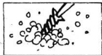
Soaping the threads makes it easier to screw a wood screw into wood.
