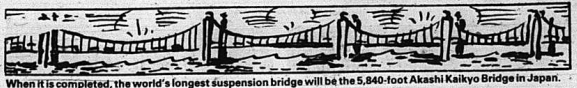
When it is completed, the world's longest suspension bridge will be the 5,840-foot Akashi Kaikyo Bridge in Japan.
