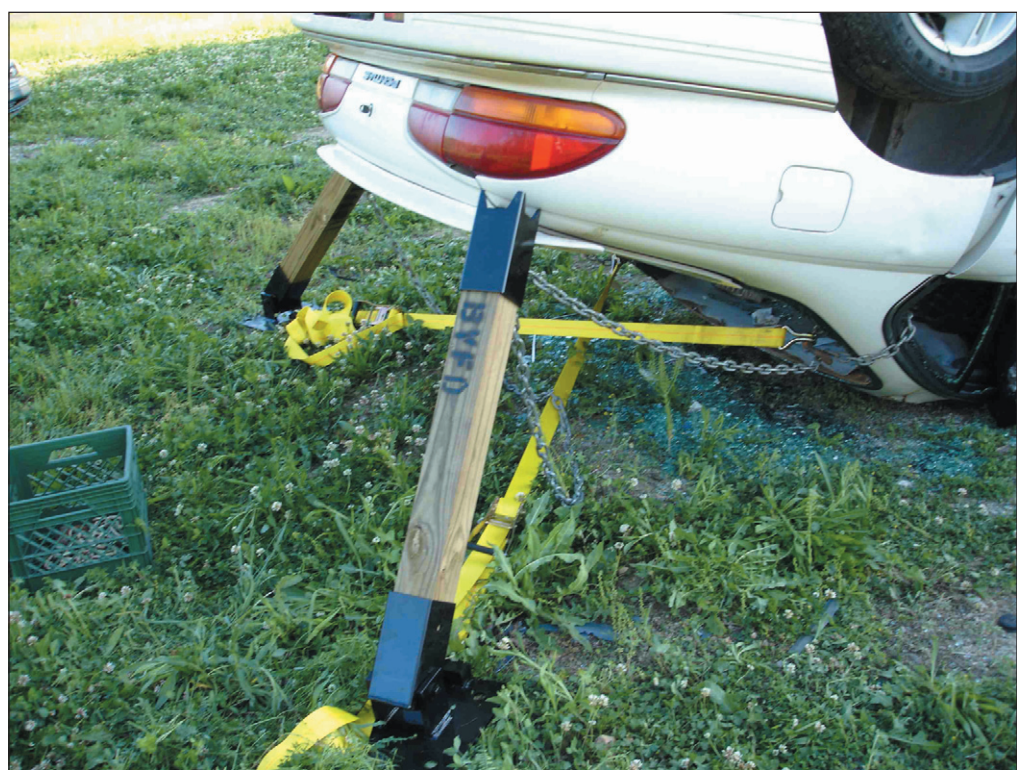
Brodhead Fire Department has added many tools to conduct rescue activities. Shown above are a strut and shoring kit used to stabilize a vehicle in a roll-over situation. The kit can also be used for structural collapse and farm equipment rescue.
