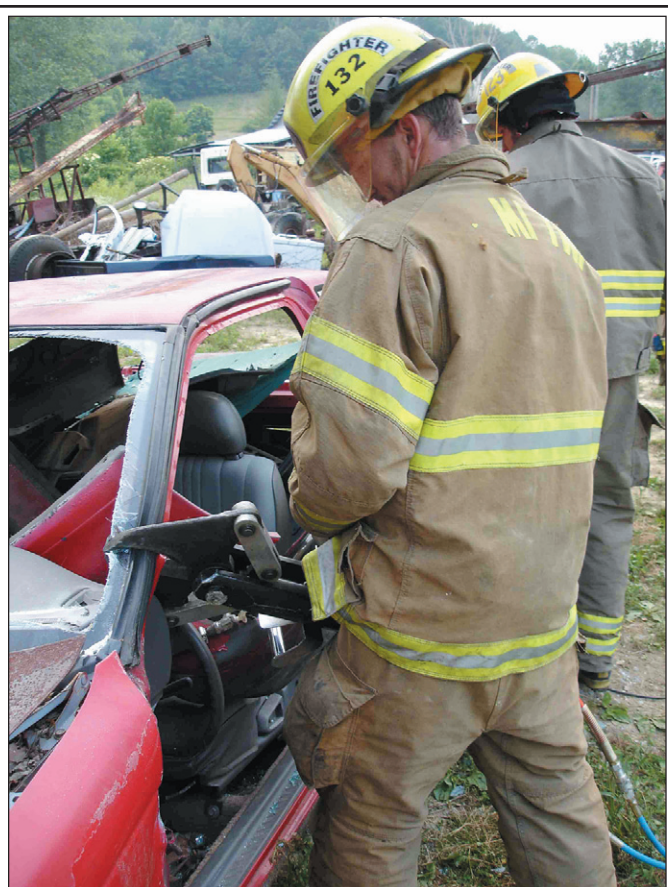
Brodhead firefighter Jon Kerns removes the front post (A post) of a car with the "Jaws of Life" cutters, in a recent training session. Countless hours of training has been spent to prepare Brodhead firefighters to effectively deal with rescue situations.
